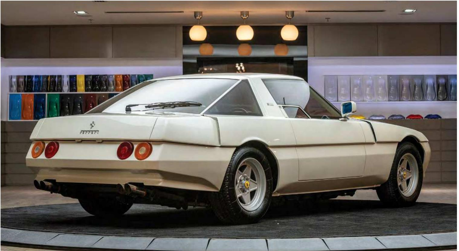
Mix of steel and aluminium in new body made it lighter than base 400i. Radical 1983 cabin (inset left) has since been altered
